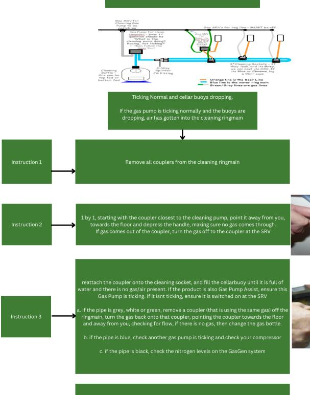
If the gas that is powering the Flowjet is coming into the system, give the pump a couple of sharp taps, on the front (but not too hard)
